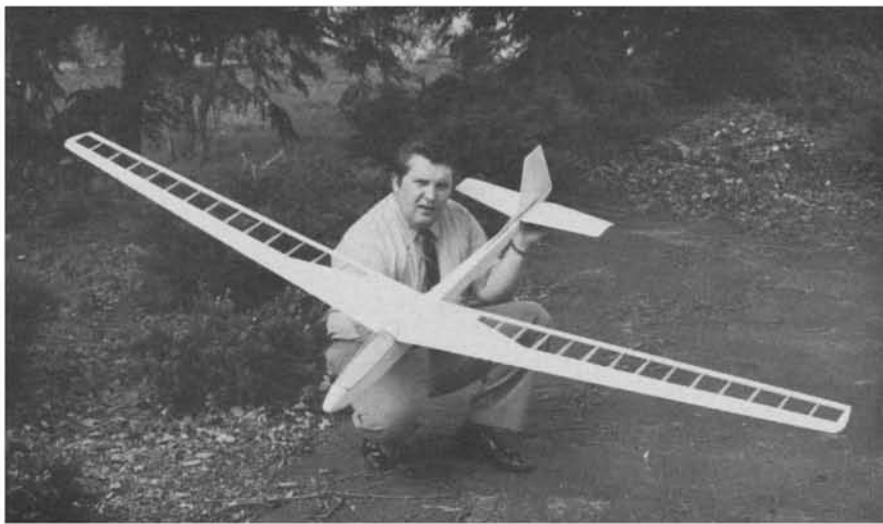
Above, Gene and the Monterey, one week after beginning assembly. Fuselage is covered and ready for painting and wings are ready for MonoKoting. Above right, electric winch launches are easy! Point nose up slightly, step on foot switch and release. Hand tows and hi-starts work well too.
